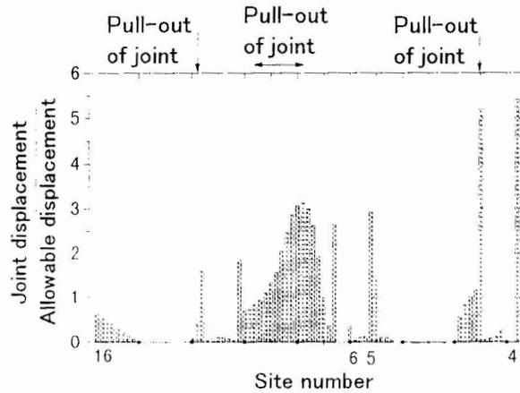
Fig. 14 Joint displacement divided by allowable value in Fukaehama.
