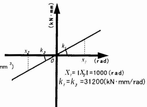
Fig. 3 Joint resistant characteristics for bending ( Mechanical joint,  $\phi 200\text{mm}$ ).
