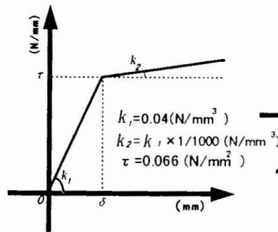
Fig. 2 Joint resistant characteristics for expansion and contraction ( Mechanical joint,  $\phi 200\text{mm}$ ).
