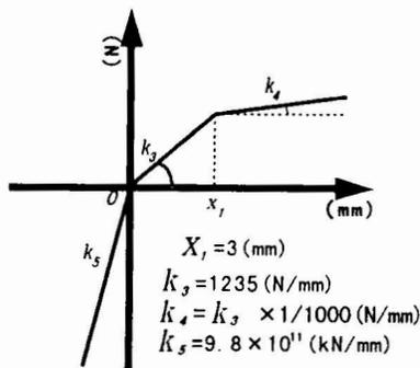
Fig. 1 Soil spring characteristics
